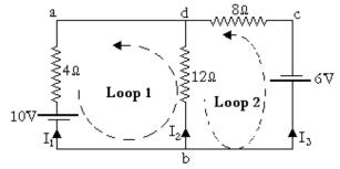
ii) Consider the circuit above. Calculate the current  $I_1$ ,  $I_2$  and  $I_3$  in the circuit of figure
